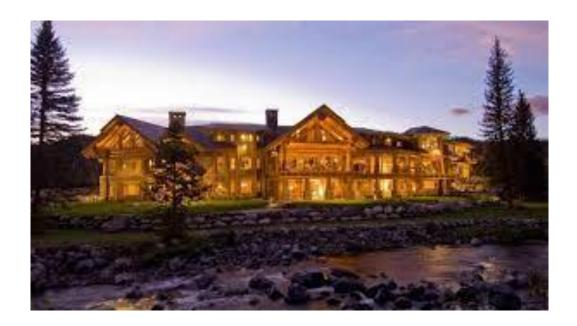
Each and every log used to build our custom Pioneer Log Home is seasoned and air dried to help control shrinking and checking. This process helps us create custom log homes that need very little adjustment and maintenance.
