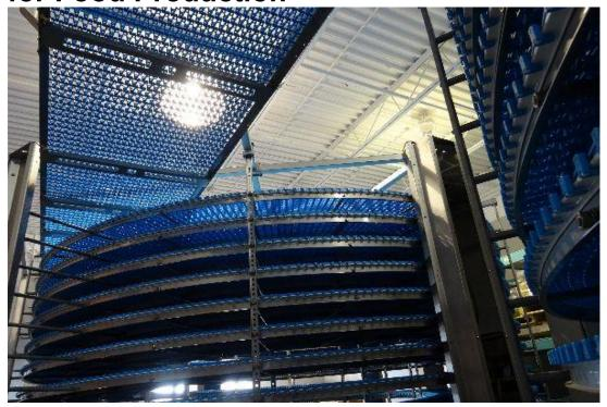
The <u>spiral conveyor</u> has become a standard across many manufacturing and production environments because of its space saving and increased production throughput abilities. But few sectors rely on them more than food and beverage production as an integral part of the cooling process.
